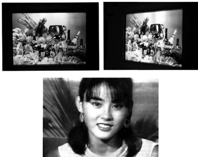
Figure 22. Two examples of AFLC display prototypes from Denso Corporation; (top) two views of a 6" screen scanning 220 lines at a refresh rate of 60 Hz demonstrated in 1993. The stated contrast ratio is 23:1; (below) video display of same size and resolution demonstrated in 1995 with a somewhat higher refresh rate and contrast 30:1. In 1998 Denso also demonstrated good 17" desktop models with 1200 lines for static pictures (though less sophisticated than the Canon displays).
