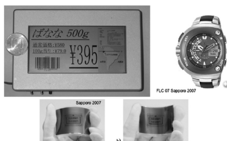
Figure 15. Some examples of hard and flexible bistable passive matrix FLC displays manufactured by Citizen. The monochrome reflective display on top left has a resolution of 1000 dpi (dots per inch). The bistability is achieved by SiO evaporation that gives a high pretilt (about 20^\circ ).
