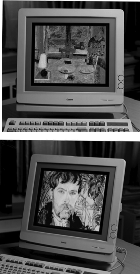
Figure 14. Canon 15 inch color screen that went into production 1995. The display has 1280 \times 1024 pixels, each divided into 4 subpixels. The cell gap is 1.1 \mu\text{m} .
